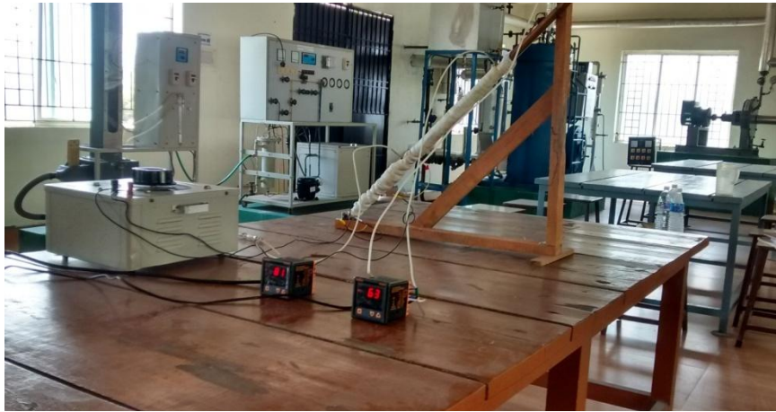
Fig. 8 Heat Pipe at 60 0 Angle of Inclination
