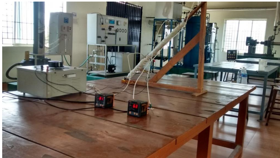
Fig 5. Heat Pipe Experimental Setup
