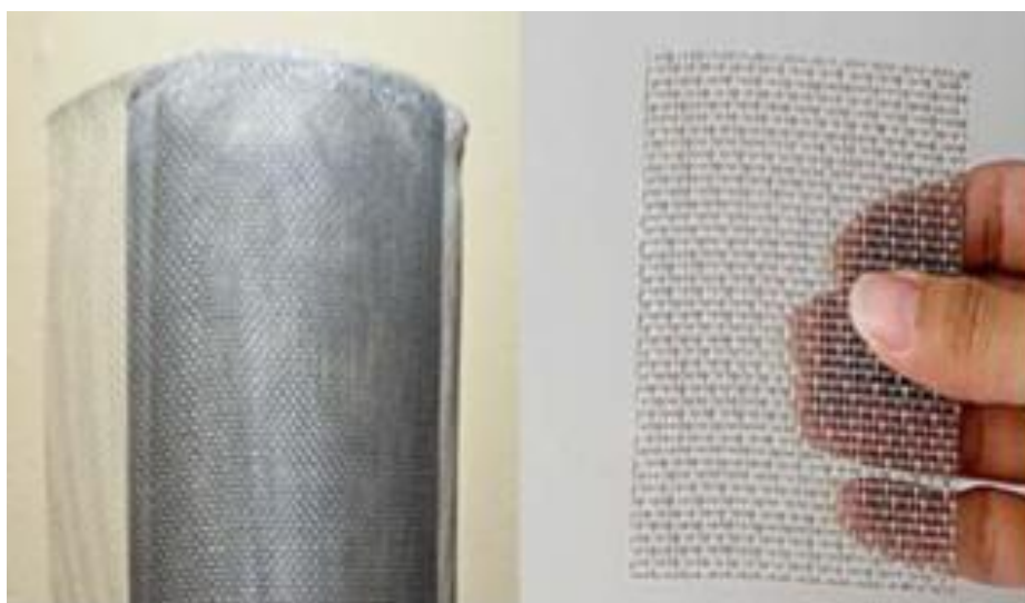
Fig .3 Screen mesh wick used in the heat pipe
